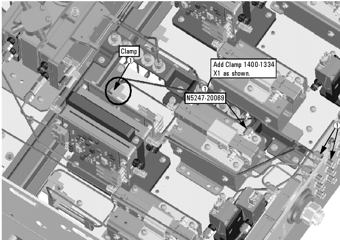
Figure 11 Location of Cable Clamp to Secure W41 (N5247-20069)
